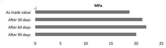
Lap shear strength versus heat ageing (ISO 4587) (typical average values)
