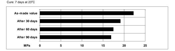
Lap shear strength versus tropical weathering (40/92, DIN 50015: typical average values)
