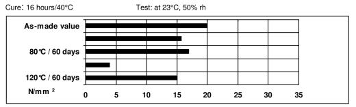
Lap shear strength versus tropical weathering (40/92, DIN 50015; typical average values) Cure:16 hours/40°C: Test at 23°C.
