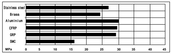
Lap shear strength versus temperature (ISO 4587) (typical average values) Cure: 1 hour at 100°C,tested at 25°C,Sand blasting steel-Sand blasting steel
