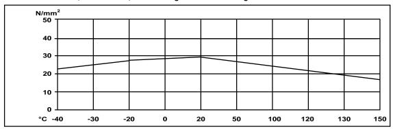
Other typical characteristics Cure: 1 hour at 100°C, tested at 25°C, Sand blasting steel-Sand blasting steel
